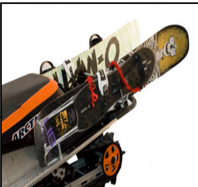
Figure 5 (8)Front Edge Guard (9)Front Peg 1.5" From this crease 1.75" From side of tunnel
