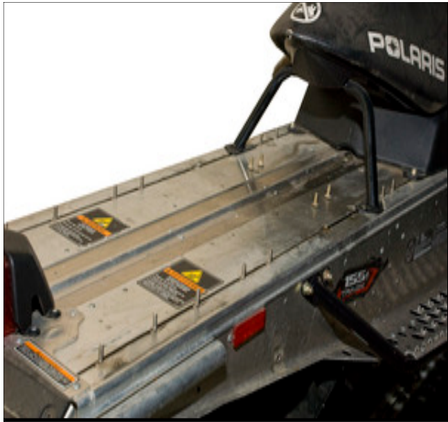
Figure 1 Carriage Bolts (7 each side, 2 between seat & seat mount brackets)
